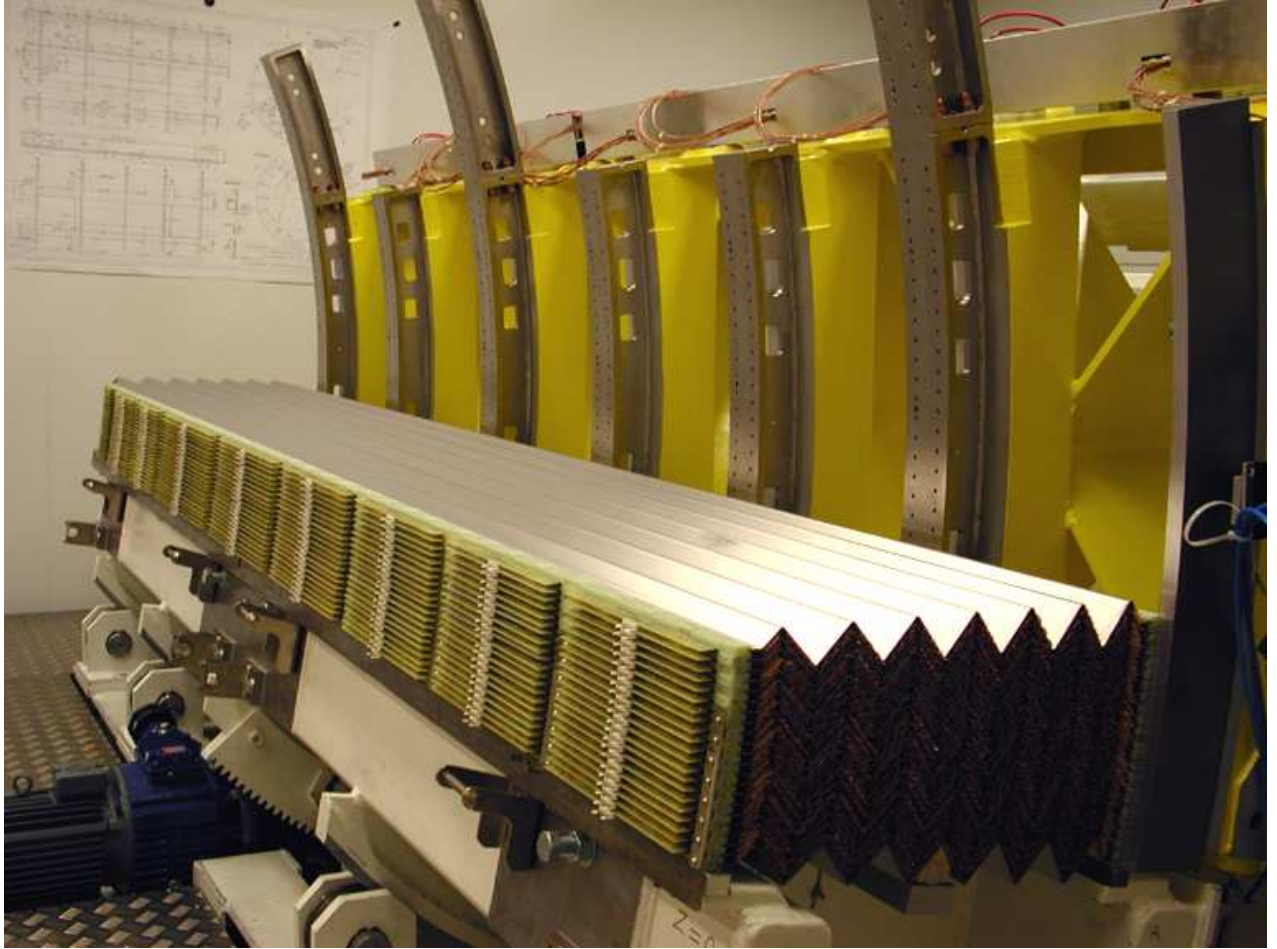
Fig. 2. One partly stacked module. The 6 outer rings on which are screwed the absorbers can be seen. Also the backbone (yellow part) and the assembling bench (white part) are visible.
