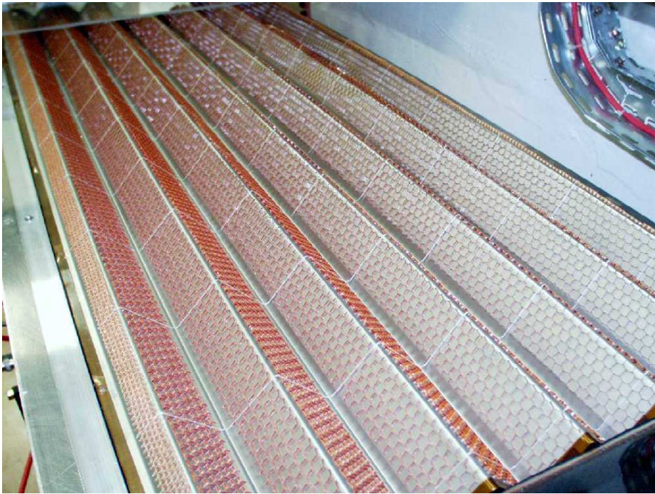
Fig. 8. One spacer resting on one absorber.
