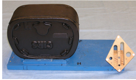
Figure 1: 3D abdominal model ("Phantom") used in the experiment (placed in ventral decubitus).
