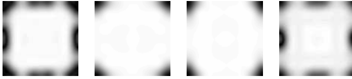
Fig. 5. Amplitude spectra of the luminance filter for each position (1, 2, 3 and 4) in the superpixel. At position 2 and 3 (G pixels), luminance can be retrieved with a maximal horizontal and vertical acuity.
