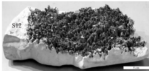
FIG. 1: Picture of a stylolite surface (S12A) in a limestone from Vercors Mountains. Magnitude of the peaks are typically of the order of 6 mm.
