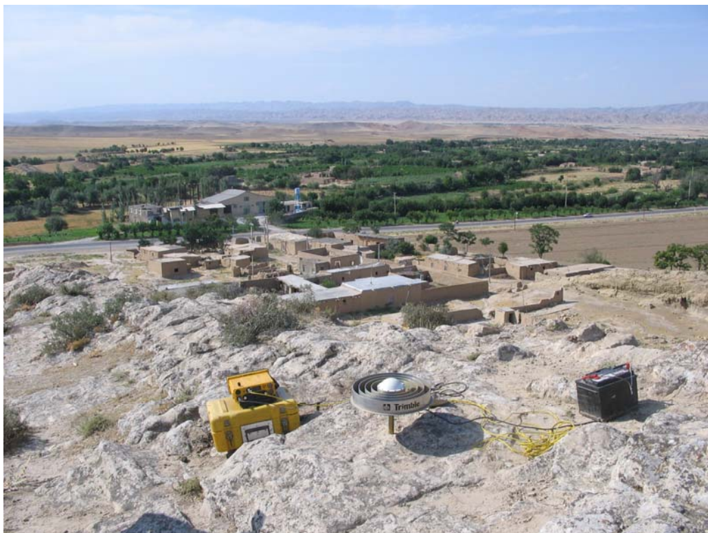
Figure 3-5. Example for a GPS station of the Kopeh Dagh network (site JANA) with forced antenna centring on bed rock.
