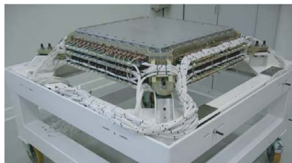
Figure 3. The calorimeter fully equipped with front-end electronics.
