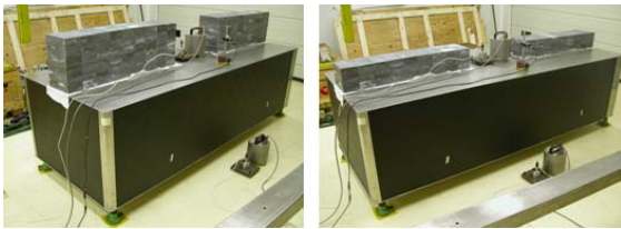
Figure 2: Honeycomb table with lead masses representing final doublets weight (1188kg) and final doublets weight / 2 (594kg)
