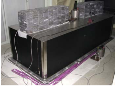
Figure 12: Honeycomb table with lead masses representing final doublets weight (1188kg)
