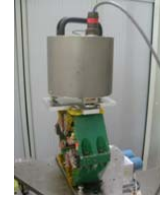
Figure 18: GURALP sensor put on the ATF2 sextupole by the intermediary of a T-plate fixed with beeswax
