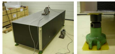
Figure 1: Honeycomb table fixed to four steel feet with adjustable height at its corners
