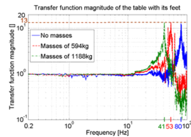
Figure 5: Transfer function magnitude of the honeycomb table with its four feet
