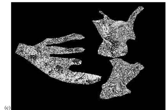
Fig. 3. Wrapped phase difference between interferograms on the Tour, Trient, and Saleina glaciers with the new DEM. (a) \Delta\Phi_{\text{April-March}} . (b) \Delta\Phi_{\text{April-December}} . (c) \Delta\Phi_{\text{April-October}} .
