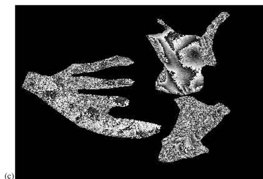
Fig. 2. Wrapped phase difference between interferograms on the Tour, Trient, and Saleina glaciers. (a) \Delta\Phi_{\text{April-March}} . (b) \Delta\Phi_{\text{April-December}} . (c) \Delta\Phi_{\text{April-October}} .
