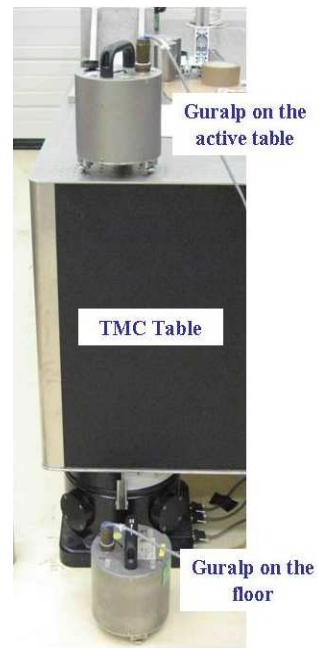
Fig 05b: Measurement set-up with a Guralp sensor placed on the active table
