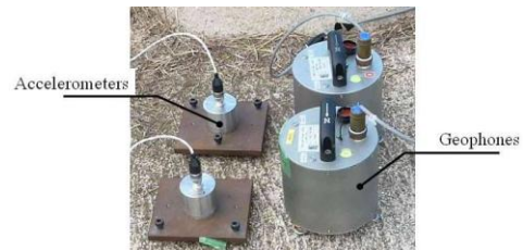
Figure 2: Layout of the set of measurements.
