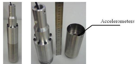
Figure 8: Developed waterproof accelerometer support.
