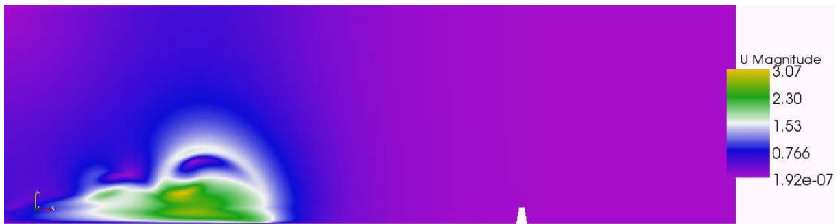
FIGURE 8. Velocity field magnitude at t = 25 s. The color scale ranges from 0 m/s to the maximum value 3.07 m/s.
