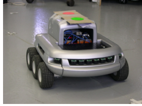
Figure 1: The Koala ® mobile robot (K-Team company), next to a volleyball, for size reference. The red and green dots on top of the robot were not used in the experiments described here.
