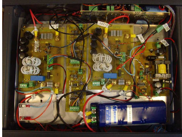
Figure 7. Arrangement of power converters in the test-bench setup
