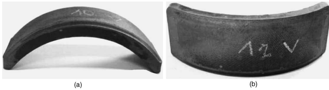
Fig. 3. Sintering positions: (a) horizontal; (b) vertical.
