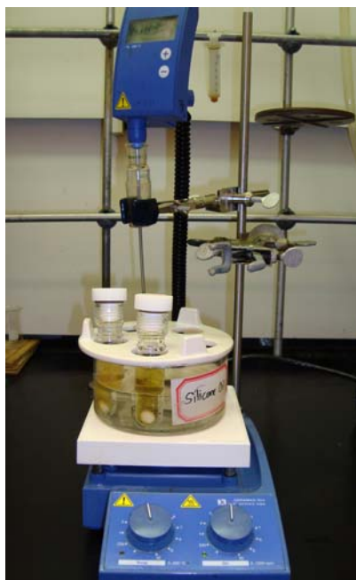
Figure 13: Reactor set up for Knoevenagel reaction
