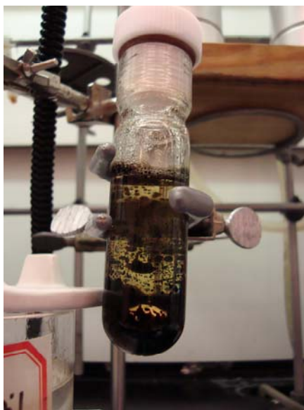
Figure 33: Picture of solid product in pressure tube after Knoevenagel reaction of HMF and malonic acid in toluene
