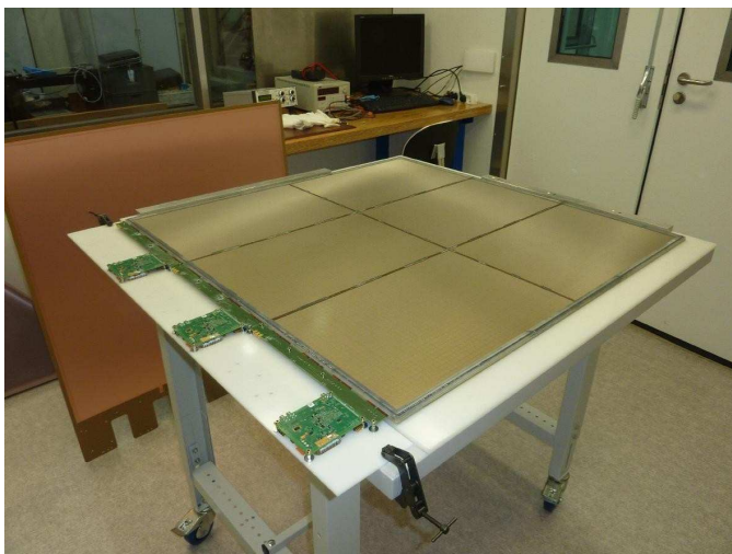
Figure 2: The 1 \times 1 \text{ m}^2 prototype during assembly showing the mesh side of the six ASUs, the readout boards and the cathode cover.
