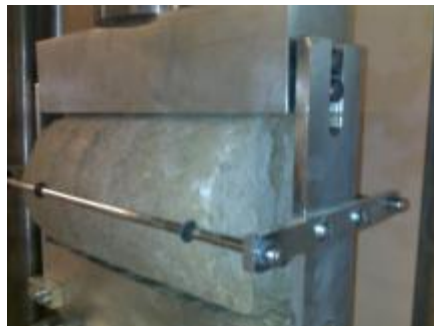
191 192 Figure 5 Brazilian test to determine the tensile strength
