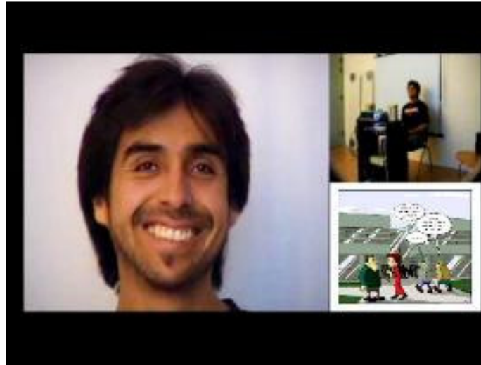
Figure 2. Three video streams gathered and mixed in real time (encoder's zoomed in face, full length and screen activity)
