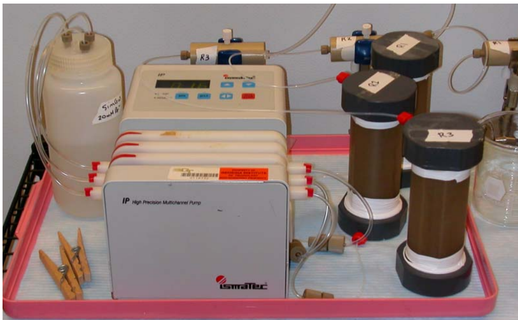
Figure 5.2. Photograph of the flow-through reactor experimental set-up showing, from left to right, the synthetic groundwater influent, multi-channel peristaltic pump, and three flow-through reactors and flow cells. A voltammetric Au/Hg microelectrode was positioned in the flow cell during oxygen measurements and the effluent was collected periodically with a fraction collector (not pictured).
