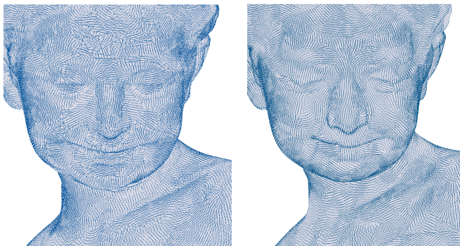
Figure 9: Principal direction estimation on Bimba datas (no noise). We put a line-segment aligned at every point to the minimal principal direction. Left: Jet-fitting method (with a polynomial of degree 4 \times 4 and k = 100 neighbors for each point). Right: d_{P,k}^w -VCM method (parameters R = 0.04D , r = 0.08D , k = 30 , where D is the diameter of the original shape.)
