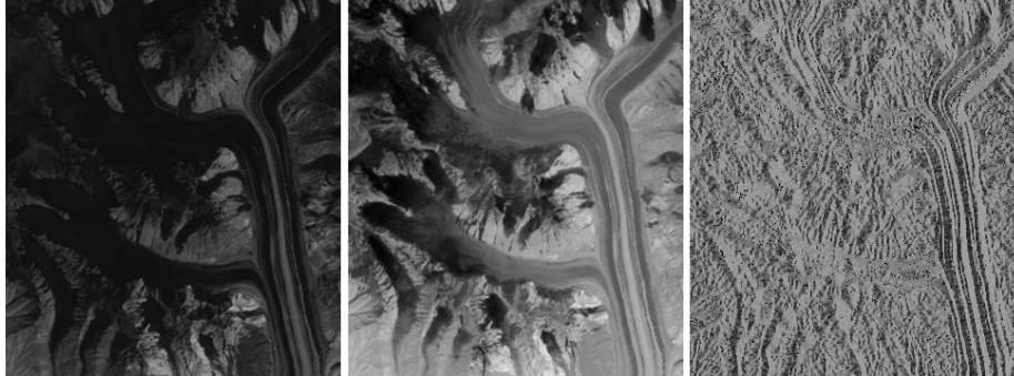
Figure 2: Example of enhancement procedure for Landsat images over northern tributaries of the Baltoro glacier (Karakoram) : Landsat mid-infrared band 5 (left) has the best performance in the Karakoram (see section 3.2.2), selecting the first component of a PCA of bands 4 & 5 results in brightening of the accumulation zones (middle), the gradient orientation displays enhanced glacier features (right).
