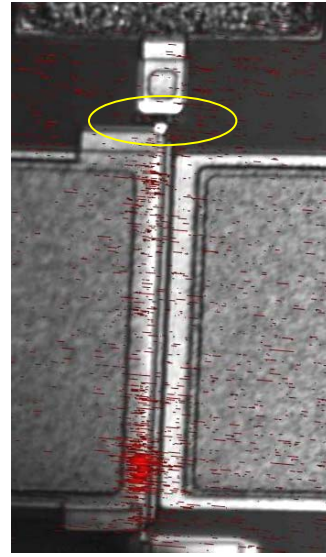
M13-site R85, X50, After FIB 1 cut Contact probe at the end of the gate finger V_{GS} = -4.89V , I_G = 420 nA
