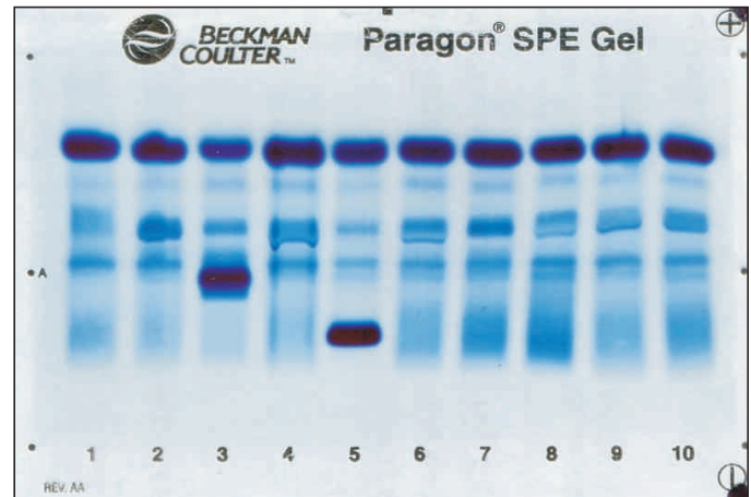
Figure 1: Serum Protein Electrophoresis on Agarose Gel Each column of the gel is representing the single sample of the patient except the first column for the control. The monoclonal gammopathy is determined by the presence of a well defined band in the beta and gamma region as seen in 3 rd and 5 th columns, respectively. Similarly the polyclonal gammopathy can be seen in the gamma region on the 8 th column of the gel. In the 6 th column hypoalbuminemia with increase in the alpha 2 fraction can be noted which may be seen in the cases of nephrotic syndrome.
