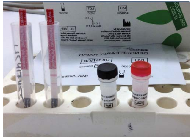
Fig. 2. Panbio Dengue Early Rapid, an immunochromatographic assay for detection of NS1 antigen Source: AKU/Binish Arif
