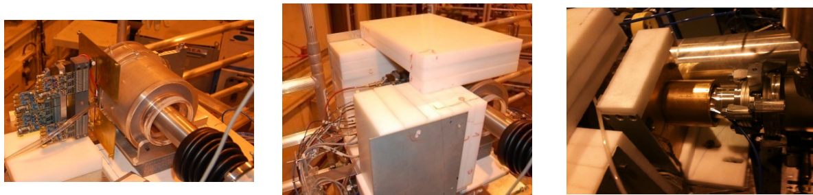
Figure 4. From left to right, sunrise micromegas in different shielding setups. Left: The detector with the lead, cadmium and copper shielding. Middle: The detector with the addition of polyethylene shielding. Right: New shielding implemented in 2011 to block an important contribution of the background events that come from the pipes.
