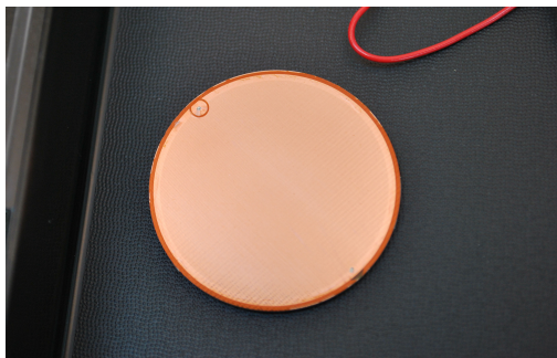
Figure 10. The first generation of microbulk Micromegas used. They had a diameter of 35 mm and an amplification gap of 50 \mu\text{m} .
