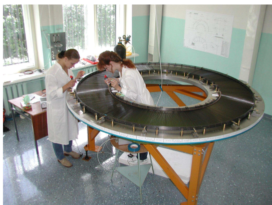
Figure 22. Gluing straws into the carbon-fibre rings.
