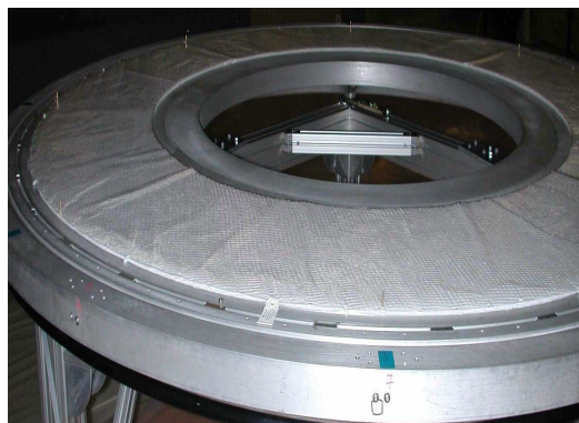
Figure 17. A radiator of an early batch showing ridges (see text).
