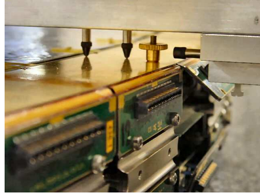
Figure 34. Digital measuring probes held by a rotary arm that are used to measure the dimensions of each eight plane wheel.
