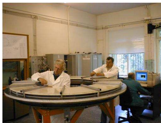
Figure 23. Four-plane wheel undergoing a gas leak measurement. The cover closes the volume between the inner and outer rings. The twelve aluminium bars which clamp the table and cover are visible.
