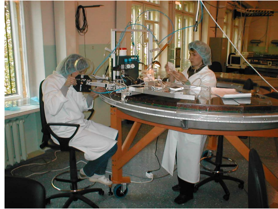
Figure 27. The four-plane wheel during wiring. The wiring machine installed above the wheel.
