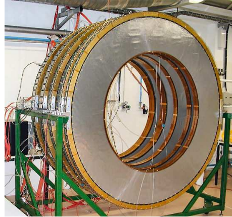
Figure 36. High voltage test stand with several end-cap wheels under high voltage.
