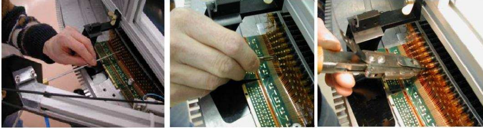
Figure 28. The nose of the feed block fitted to blow the wire through the straw by the air stream (left). Insertion of the outer crimping pin into the hole of the HV plug (center). Wire crimping using the in-house fabricated pneumatic crimp tool (right).
