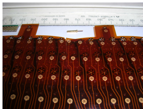
Figure 4. The flexible layers of a Wheel End-Cap Board (WEB) with the conductive paths for a signal from anode wires to the rigid part of the board. The anode wires are connected to the path via a crimping pins (one seen on the photo) through holes with six inward-pointing petals.
