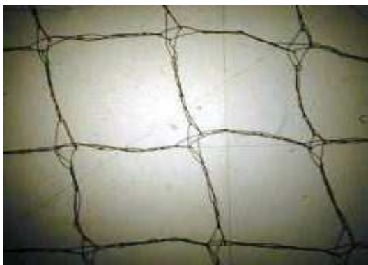
Figure 16. Picture of the type-A spacer fabric used for the TRT end-cap radiators.
