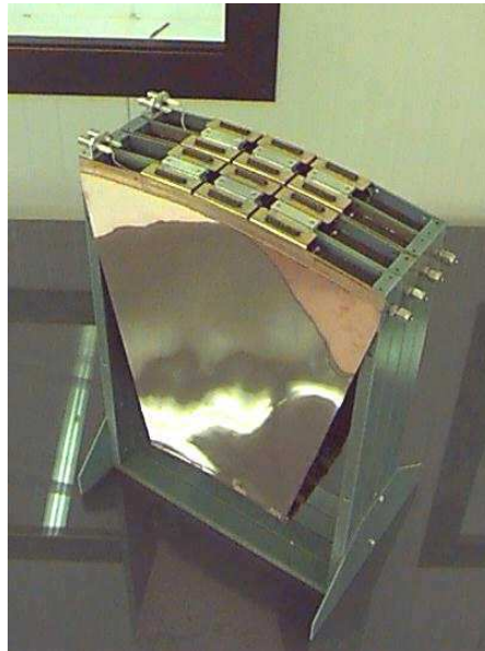
Figure 62. The TRT end-cap test beam prototype representing one sector of the 16 plane wheel.
