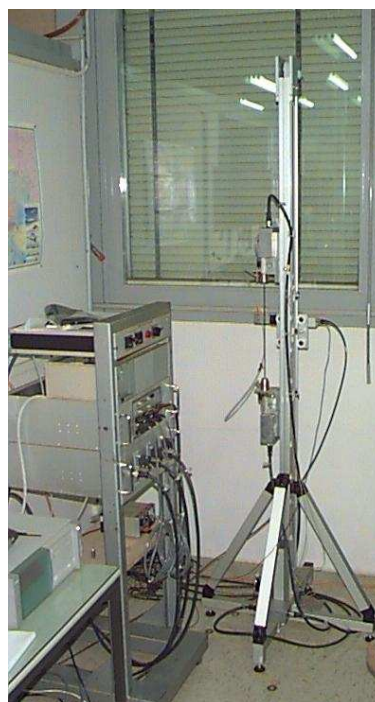
Figure 8. The machine measuring straw straightness and length.
