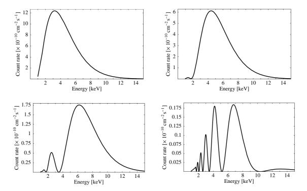
Figure 4: Expected photon spectra depending on the shift  $S = m_{\gamma} - m_a$  from the resonance: S = 0 (top left), S = FWHM/2 (top right), S = FWHM (bottom left)  $S = 3 \times \text{FWHM}$  (bottom right). An axion-photon coupling constant of  $1 \times 10^{-10}$  GeV<sup>-1</sup> is assumed.
