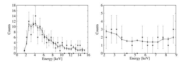
Figure 5: Energy distribution of events recorded during the tracking run (stars with dashed line) at pressure setting  $P_k = 8.909$  mbar compared to background data (empty squares with continuous line) for the TPC (left) and the Micromegas (right) detectors respectively.
