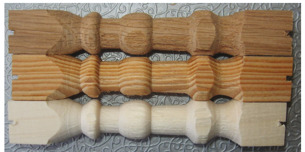
Figure 3. Turning test specimens (sessile oak, European black pine, black poplar).
