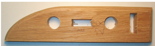
Figure 2. Test specimen (sessile oak) that is shaped, bored, and mortised.
