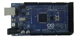
Fig. 9 Arduino Microcontroller Board
