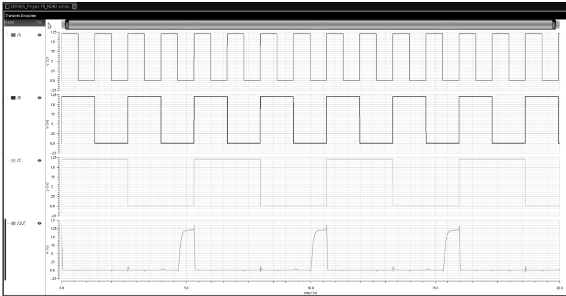
Fig. 40: Transient response NOR3.
