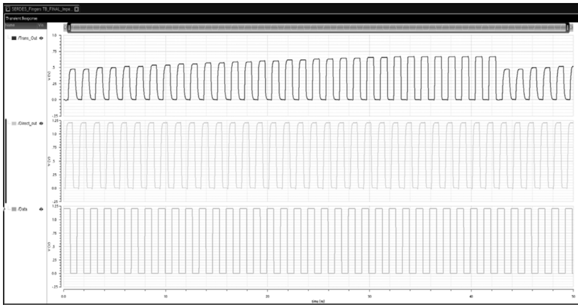
Fig. 70: Transient response for Impedance of Transmitter module based on its transistor level version.
