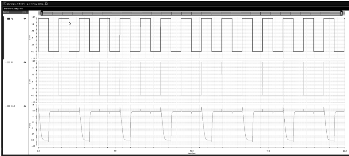
Fig. 38: Transient response of NAND2.
