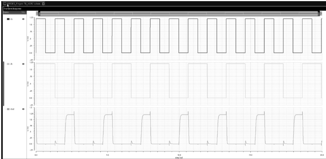
Fig. 36: Transient response of NOR2.
