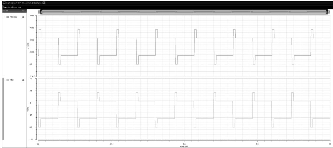
Fig. 15: Transient response for Pre emphasis of Transmitter module based on its macromodel.
