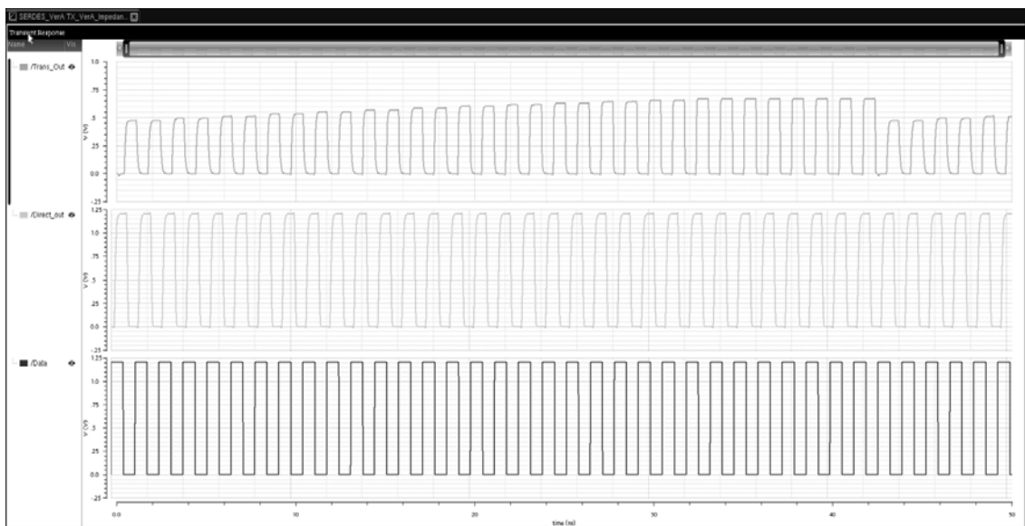
Fig. 71: Transient response for Impedance of Transmitter module with Decoder 4-12 Verilog-A module.
