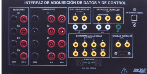
Fig. 5. Data acquisition and control module.
