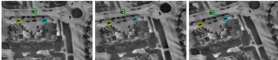
Figure 2. Tracking results from two algorithms on six consecutive frames from the IR Traffic sequence. These videos were tracked at a reduce frame rate of 5fps. These frames were selected because of the large rotational camera motion present. (a): Failure to track by mean-shift localization with a Kalman filter modeling coupled motion. The targets found in the final frame are not the original targets. (b): Successful tracking by proposed method with decoupled camera and target motion models.
