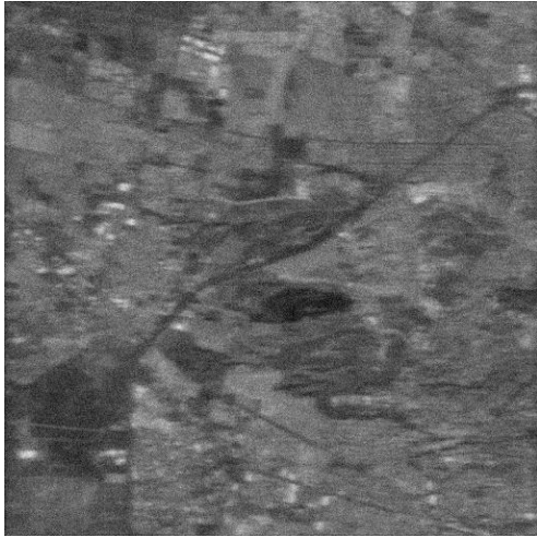
Fig. 2. Enhanced radar image formed applying the descriptive constrained least squares (CLS) algorithm.
