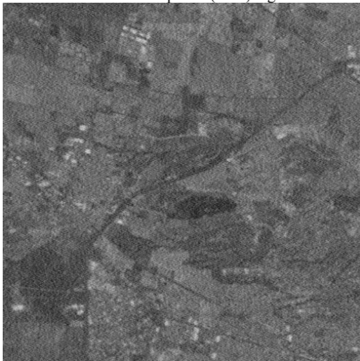
Fig. 4. Enhanced radar image formed applying the modified descriptive weighted constrained least squares (WCLS).
