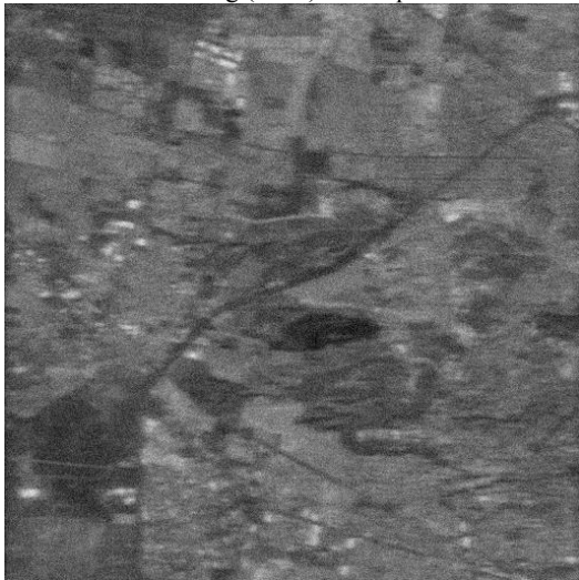
Fig. 3. Enhanced radar image formed applying the descriptive constrained least squares (CLS) algorithm.
