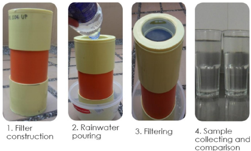
Figure 32. Filter materials testing procedure.
