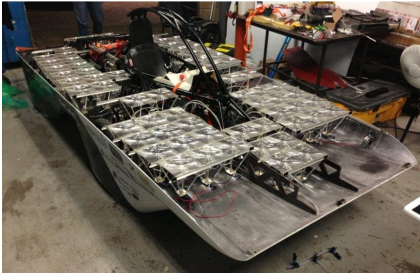
Figure 11. Exposed CPVs assembled in Primavera solar car.
