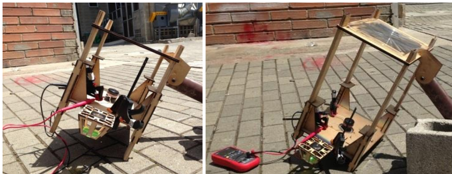
Figure 6. Device designed to experimentally find the most suitable distance between a Fresnel lens and a photovoltaic cell.
