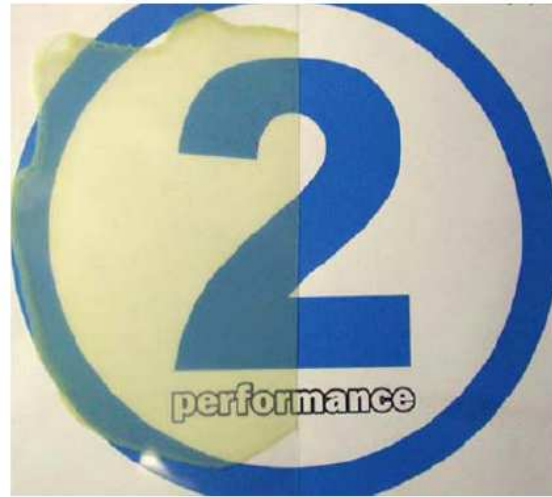
Figure 2.20. Image demonstrating the transparency of an ITO-PVP nanocomposite film. [72]
