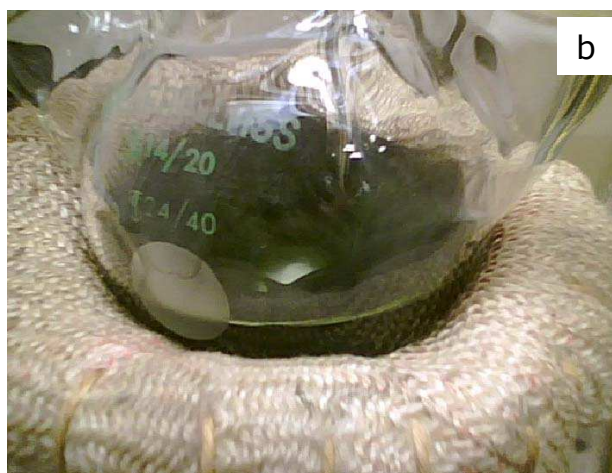
Figure A.1. (a) Schematic of custom-made apparatus designed for the synthesis of colloidal ITO nanoparticles; (b) Image of colloidal ITO nanoparticles synthesized in reaction flask over the heating mantle.
