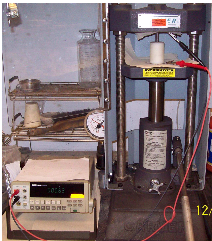
Figure 3.3. Image of experimental set up used to measure the dc electrical conductivity of ITO nanoparticle fillers.
