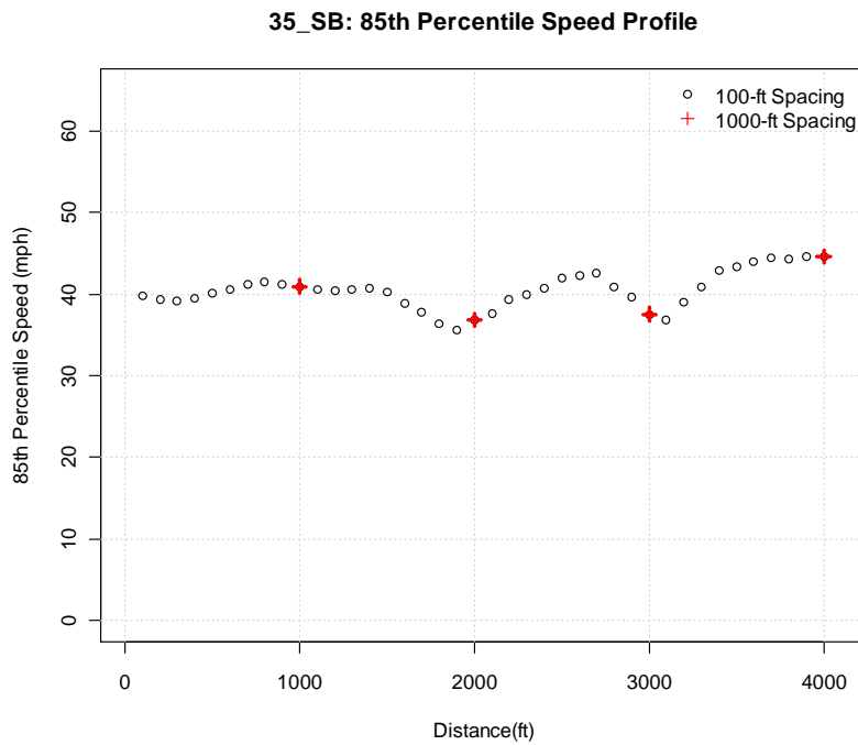
Figure 31: Profile of the 85 th Percentile Speed on the Corridor ID 35 Southbound using 100-ft and 1000-ft Sampling Distances
