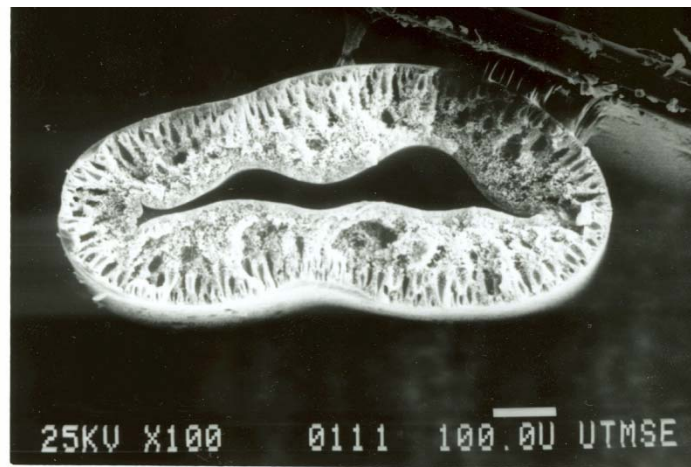
Figure 2.6: SEM picture showing the fiber collapse at high pressures due to the presence of macrovoids.[12]
