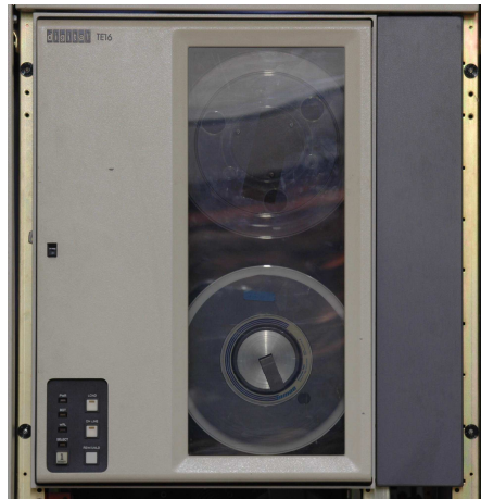
Figure 9: Nine-track tape drive
