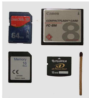
Figure 17: Selection of flash memory devices positioned next to a match for size comparison
