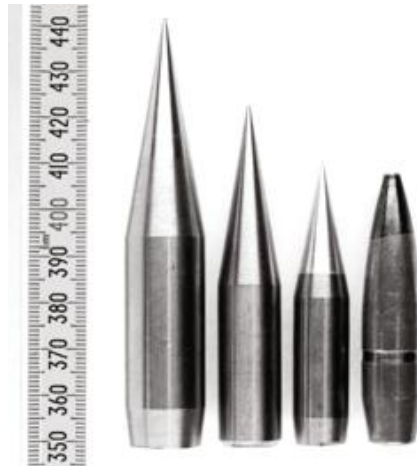
Figura 5. Municiones de armas pesadas, de izquierda a derecha, 30mm, 25mm, 20mm y 12,7mm (Fuente: Impact Engineering of Composite Structures de International Center for Mechanical Science, CISM Course and Lectures, vol. 526)
