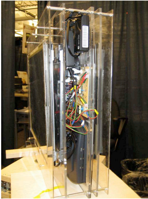
Figure E.9 This shows the construction of the spinning screen with a wireless VGA kit. The wireless VGA enables to transmit the video signal to two monitors in the upper part. This spinning screen is designed for the Steelcase spinning screen design in In-Space project at Synlab
