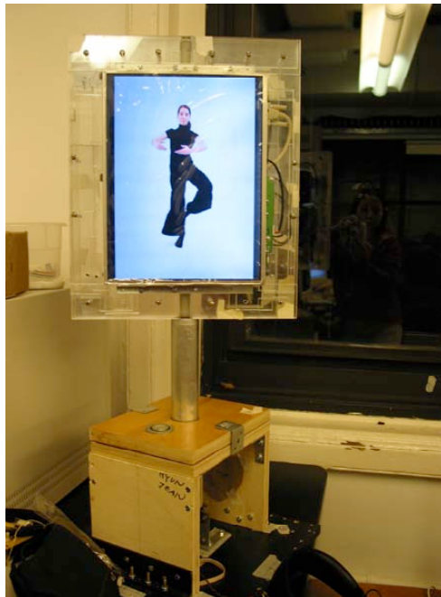
Figure E.5 and FigureE.6. The spinning screen construction testing LCD display output on one side of the screen
