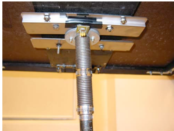
Figure B.2 A tabletop with a spring joint and an accelerometer
