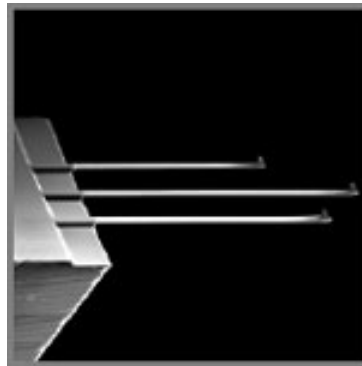
Figure 3.3. SEM image of a three-beam cantilever (CSC-38). During nanocoil attachment, one or more tips will become modified. This is due to limited control of the attraction of nanocoils to the different cantilever beams.
