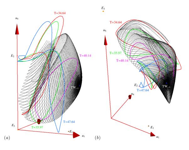
Figure 34: Two different projections of L=22 Kuramoto-Sivashinsky dynamics on invariants given in Table 4. We plot a few selected relative periodic orbits and part of the unstable manifold of  $TW_{-1}$  in black, with trajectories originating along the eigenspace corresponding to  $\lambda^{(1)}$ .
