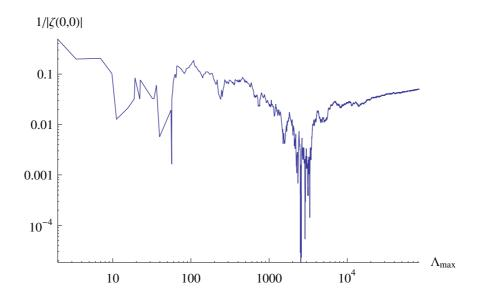
Figure 36: Consistency check of flow conservation relation (132) for Kuramoto-Sivashinsky equation (65) for L=22. Here the dynamical zeta function  $1/\zeta(0,0)$  was evaluated from (132) with stability cutoff  $\Lambda_{\text{max}}$  as in (131). The maximum stability cutoff shown corresponds to using the 5000 least unstable cycles (periodic orbits and relative periodic orbits) in the set.
