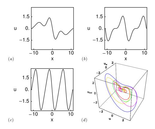
**Figure 19:** (a)  $E_1$ , (b)  $E_2$ , and (c)  $E_3$  equilibria. The  $E_0$  equilibrium is the u(x) = 0 solution. (d)  $(u, u_x, u_{xx})$  representation of (red)  $E_1$ , (green)  $E_2$ , (blue)  $E_3$  equilibria, (purple)  $TW_{+1}$ , and (orange)  $TW_{-1}$  relative equilibria. L = 22 system size.
