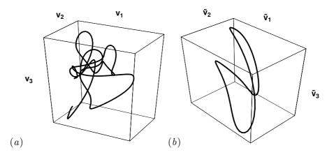
**Figure 32:** The relative periodic orbit with  $(T_p, \ell_p) = (33.5, 4.04)$  from Figure 29 (c) which appears well embedded within the turbulent flow: (a) A stationary phase space projection, traced for four periods  $T_p$ . The coordinate axes  $v_1$ ,  $v_2$ , and  $v_3$  are those of Figure 24; (b) In the co-moving mean velocity frame, traced for one period  $T_p$ .
