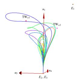
Figure 33: Phase space portrait of L=22 Kuramoto-Sivashinsky dynamics projected to invariants given in Table 3. The trajectories shown are 20 short relative periodic orbits.
