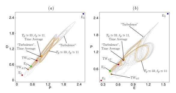
**Figure 30:** (a) Power input P vs. dissipation rate D (b) energy E vs. power input P, for several equilibria and relative equilibria, a relative periodic orbit, and a typical 'turbulent' long-time trajectory. System size L=22.
