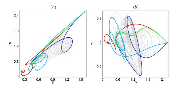
**Figure 31:** Two projections of the  $(E, P, \dot{E})$  representation of the flow.  $E_1$  (red),  $E_2$  (green),  $E_3$  (blue), heteroclinic connections from  $E_2$  to  $E_3$  (green), from  $E_1$  to  $E_3$  (red) and from  $E_3$  to  $E_2$  (shades of blue), superimposed over a generic long-time 'turbulent' trajectory (grey). System size L = 22.
