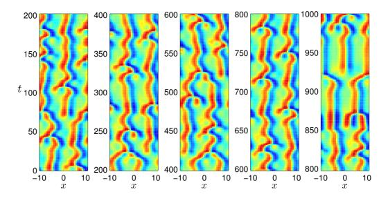
Figure 18: A typical chaotic orbit of the Kuramoto-Sivashinsky flow, system size L=22.
