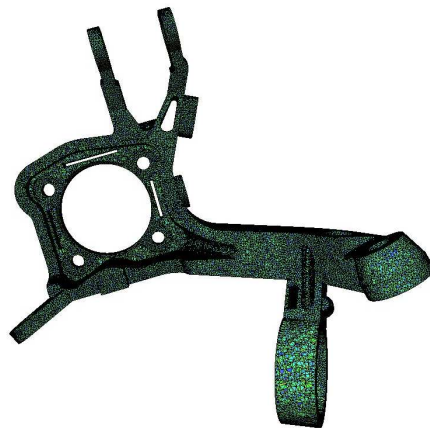
Figure 1.16: Stub axle [18]. Colormap according to the quality of the triangles
