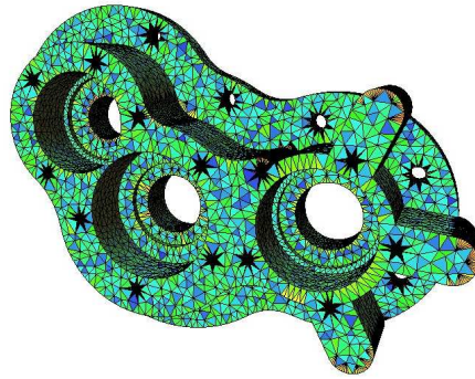
Figure 1.10: Pump carter [17]. Colormap according to quality of triangles.
