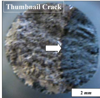
Figure 6-4: Thumbnail crack in a smooth specimen subjected to OP TMF with \Delta\epsilon_{mech}=1.26\% and T=500^{\circ}\text{C}\leftrightarrow 950^{\circ}\text{C} .
