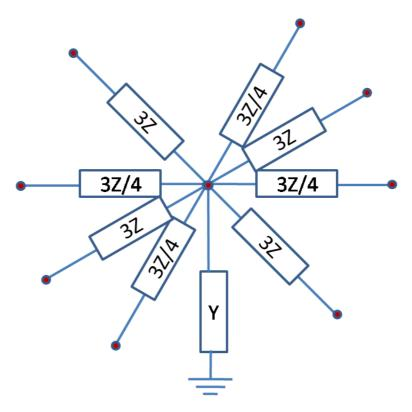
Figure 22. Unit-cell model using 9-Point Approximation (X-Unit cell).
