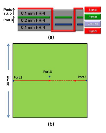
Figure 108. (a) Cross-section and (b) layout of microstrip transition.
