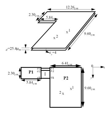
Figure 12. Segmentation of an L-shaped plane-pair.
