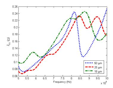
Figure 128. Self impedance at Port 1 after optimization.
