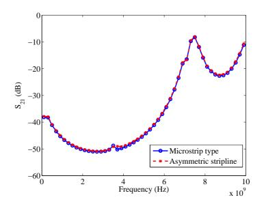
Figure 82. Insertion loss of structure in Figure 79(c).
