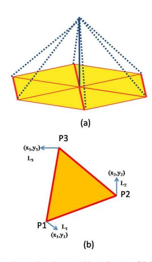
Figure 131. (a) Triangular mesh and pyramid basis function (b) Cartesian and Simplex coordinates.
