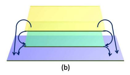
Figure 41. (a) Fringing fields due to narrowing of PDN (b)Fringing fields at edges in multi-layer geoemtries.
