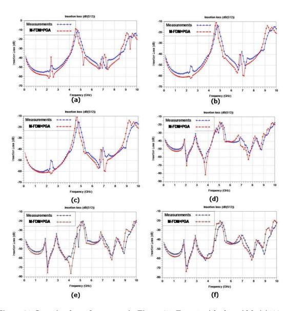
Figure 86. Insertion loss of structure in Figure 85; Type 1 with slot width (a)100  $\mu m$  (b)200  $\mu m$  (c)300  $\mu m$ ; and Type 2 with slot width (a)100  $\mu m$  (b)200  $\mu m$  (c)300  $\mu m$ .
