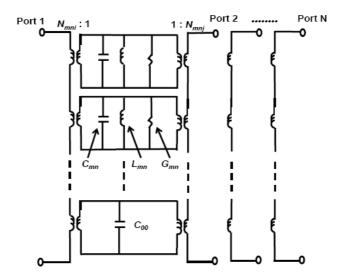
Figure 11. Equivalent circuit for a plane-pair.
