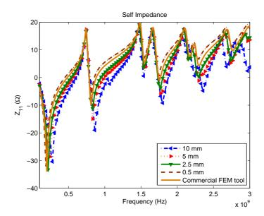
Figure 25. Self impedance,  $Z_{11}$ , with increasing mesh refinement.
