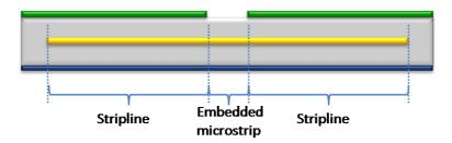
Figure 101. Stripline to embedded microstrip transition.
