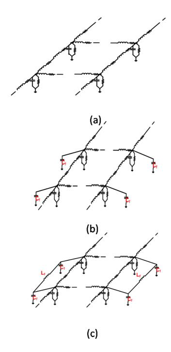
Figure 51. Addition of Fringe elements for single plane-pair structures. Equivalent circuit (a) from uncorrected M-FDM (b) upon addition of fringe capacitance (c) upon further addition of fringe inductance.
