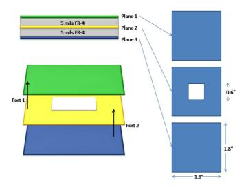
Figure 33. Test vehicle 1 (a) Geometry (b) Stack cross-section.
