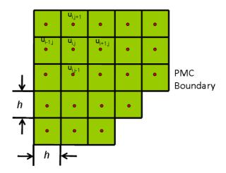
Figure 20. Discretization of the Laplace operator.
