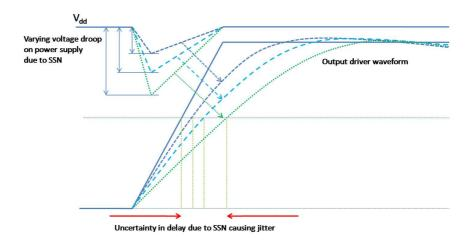
Figure 6. SSN induced jitter (courtesy [1]).
