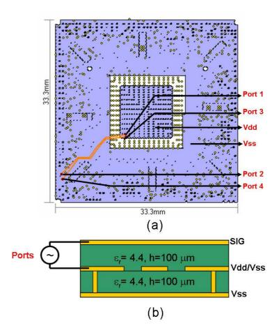
Figure 105. (a) Top view of example showing locations of ports (b) Cross section.
