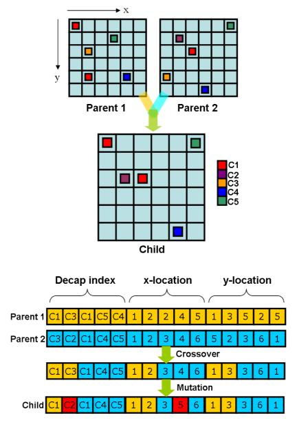
Figure 120. Schematic Illustration of Crossover and Mutation.
