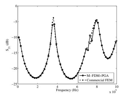
Figure 81. Insertion loss of structure in Figure 79(b).
