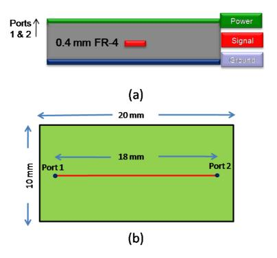
Figure 112. (a) Cross-section and (b) layout of stripline.
