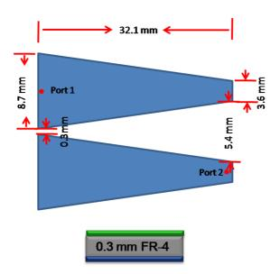
Figure 75. Geometry of coupled tapered lines.
