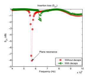
Figure 104. Insertion loss results for structure in Figure 103.
