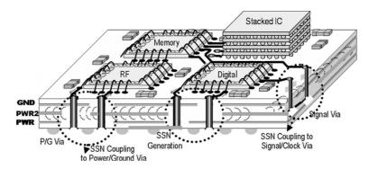
Figure 1. A System on Package Module (courtesy [2]).
