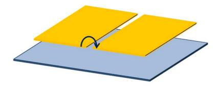
Figure 42. Gap coupling across slots in planes.
