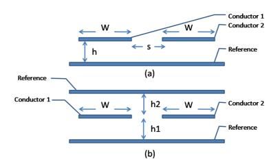
Figure 61. Gaps in Power Planes (a) Microstrip type gap (b) Stripline type gap.
