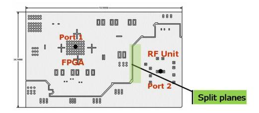
Figure 62. Mixed signal board.
