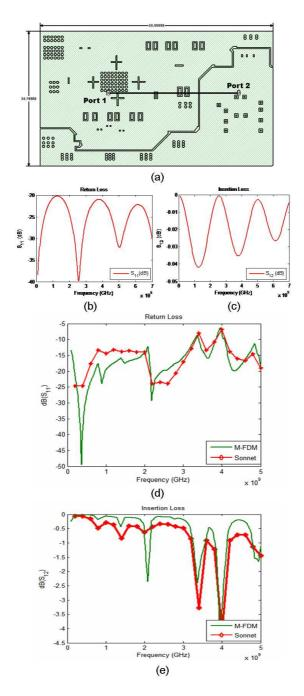
Figure 102. (a) Mixed signal board with transmission line traversing a slot (b) Return loss results - Ideal Microstrip (c) Insertion loss results - Ideal Microstrip (d) Return loss results (e) Insertion loss results.
