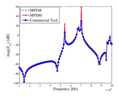
Figure 140. Magnitude of the transfer impedance  $(Z_{12})$ .
