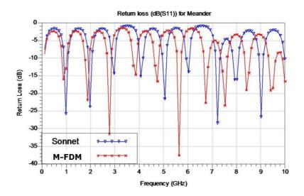
Figure 46. Return Loss (dB) of structure in Figure 45.
