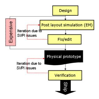
Figure 4. Current design flow.
