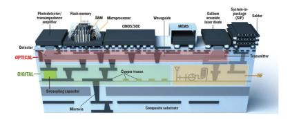
Figure 3. Schematic of a system on package (courtesy [2]).
