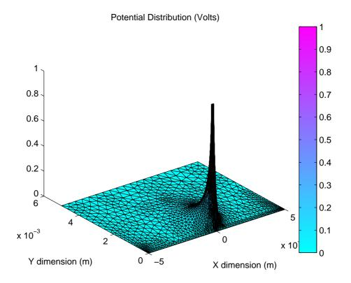
Figure 49. Potential distribution of microstrip in Figure 48.
