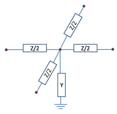
Figure 21. Unit-cell model using 5-Point Approximation (T-Unit cell).
