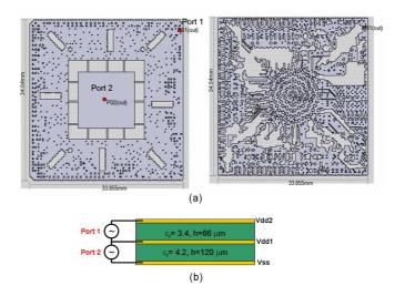
Figure 39. (a) Layouts for two package layers. Dimension is  $34\text{mm} \times 34\text{mm}$ . (b) Cross-section for the three layer example.
