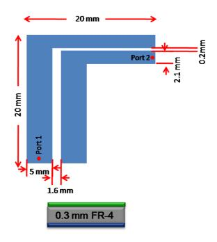
Figure 72. Geometry of coupled lines with a bend.
