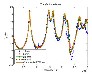
Figure 26. Transfer impedance,  $\mathbb{Z}_{21}$ , with increasing mesh refinement.
