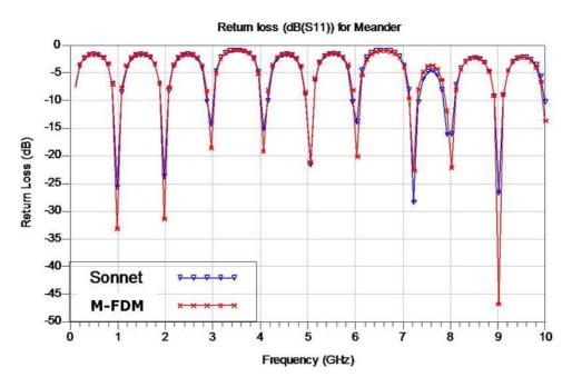
Figure 54. Return loss (dB) for structure in Figure 45 with fringe models.
