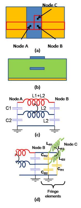
Figure 53. Addition of Fringe elements. (a) Top view of top and middle layers (b) Cross section (c) M-FDM circuit model between Nodes A and B (d) Circuit model as a result of fringe augmentation (FA).
