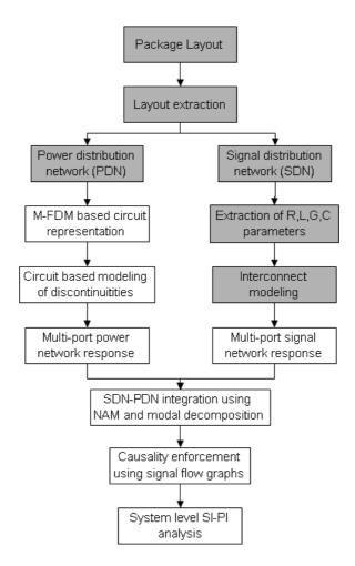
Figure 92. Proposed methodology for system level SI-PI analysis.
