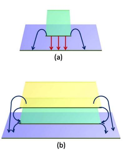
Figure 43. (a) Fringing fields due to narrowing of PDN (b) Fringing fields at edges in multi-layer geoemtries.
