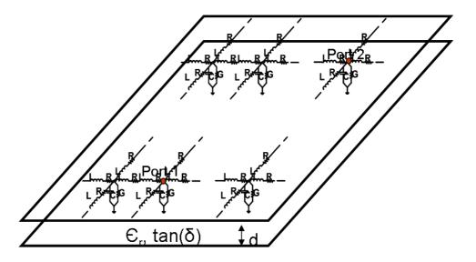
Figure 23. Electrical model for a plane-pair.
