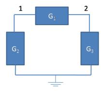
Figure 14. Simple circuit containing conductances.
