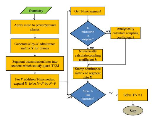
Figure 100. Flowchart for integrating transmission lines with M-FDM.
