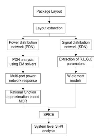
Figure 16. Flowchart for system level SI-PI analysis.
