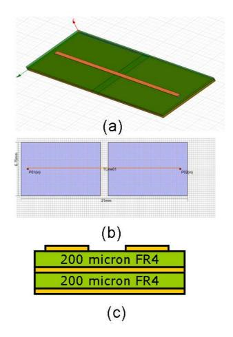
Figure 103. Top view of test case. Microstrip interconnects ports 1 and 2.
