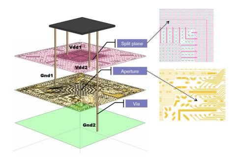
Figure 7. SSN coupling mechanisms in a realistic package.
