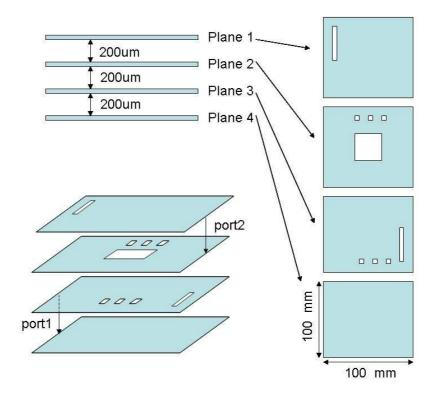
Figure 135. Four-plane test structure: cross section, location of ports, and top view of each plane.
