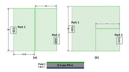
Figure 85. Manufactured test vehicles with variable slot widths (a)Type 1 and (b)Type 2.
