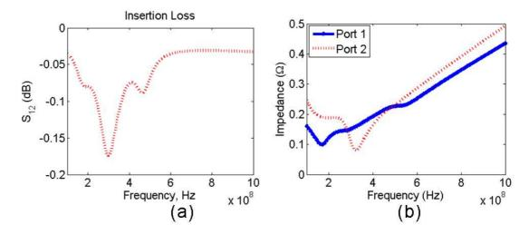
Figure 123. (a) Insertion loss of transmission line, and (b) Impedance looking into PDN at port locations in Figure 122.
