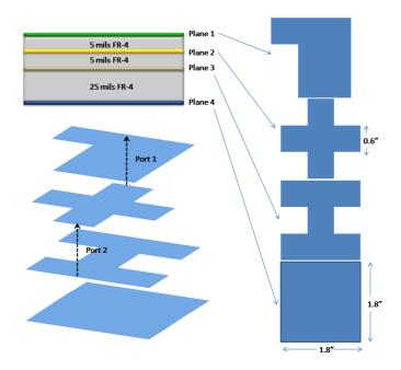
Figure 36. Test vehicle 2 (a) Geometry (b) Stack cross-section.
