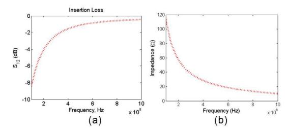
Figure 121. (a) Insertion loss of transmission line, and (b) Impedance looking into PDN at port locations in Figure 103.
