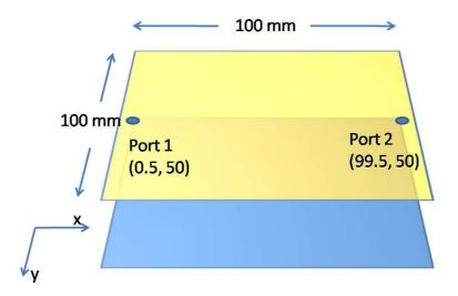
Figure 24. Geometry of test case.
