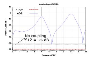
Figure 64. Insertion loss results for structure shown in Figure 63.
