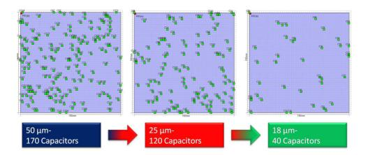
Figure 129. Locations of Decoupling Capacitors.
