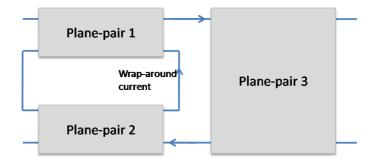
Figure 27. Equivalent network model of geometry in Figure 19.
