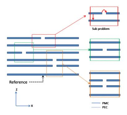
Figure 70. Multilayer geometry with multiple slots.
