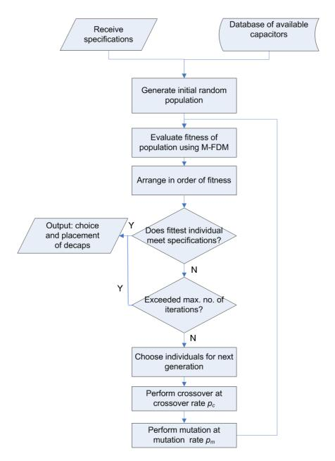
Figure 119. The flow of the GA based optimizer.
