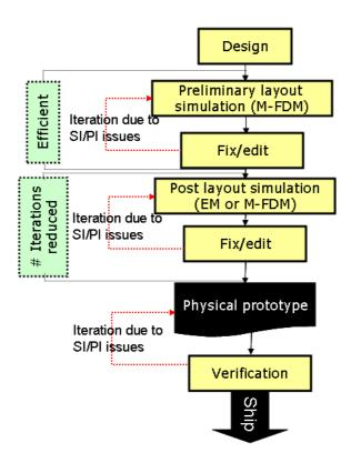
Figure 5. Efficient design flow.
