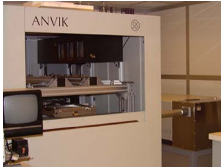
Figure 4.15 Scanning Projection Lithography/Ablation System with a 308nm Excimer Laser
