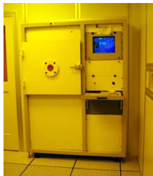
Figure 5.4 Plasma Etching System (Plasma Etch BT-1) for 300mm x 300mm substrates
