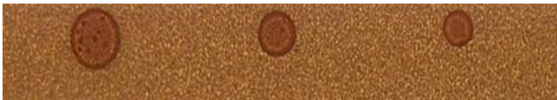
Figure 4.29 Three Different Via Sizes Ablated at Identical Conditions showing correlation between via size and amount of cones formed
