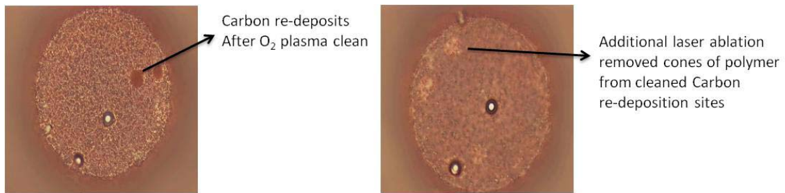
Figure 4.27 Carbon re-deposits removed by O 2 plasma clean (left) and after subsequent ablation (right)
