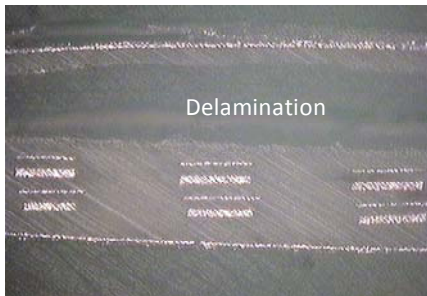
Figure 3-17. Delamination due to Insufficient Melting of LCP at 260-270°C
