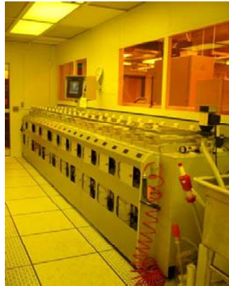
Figure 5.17 Advanced Electroless Copper Plating System with Pd Activation
