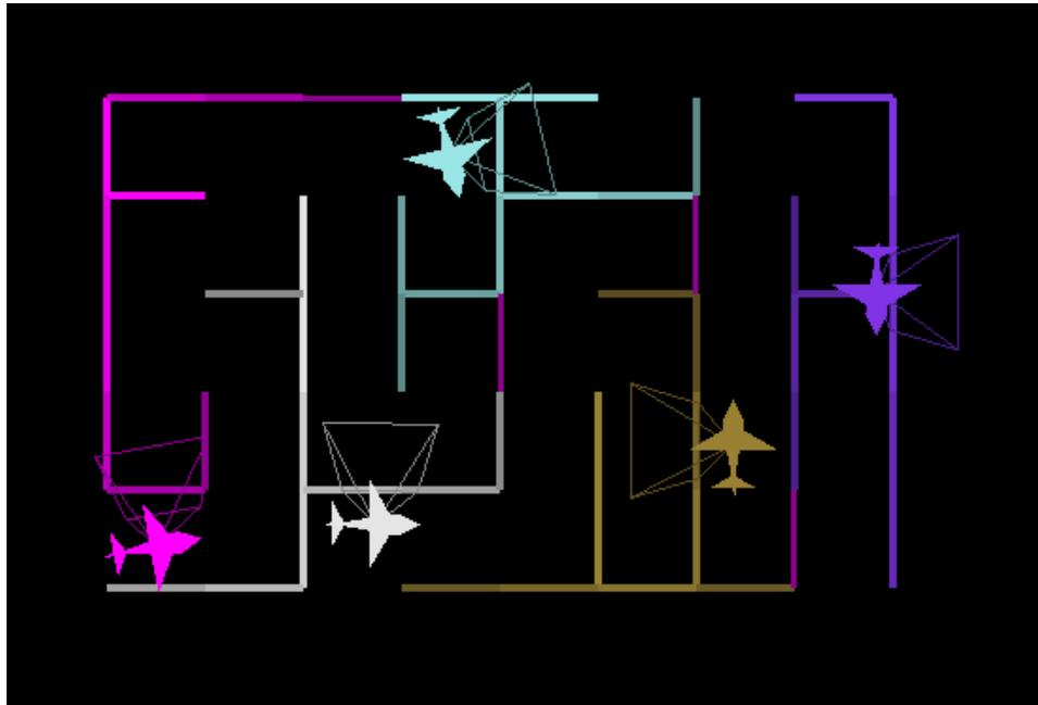
**Figure 45:** Simulation of five UAVs over a small area showing the color coded spanning trees, bridge connections, and camera projections.
