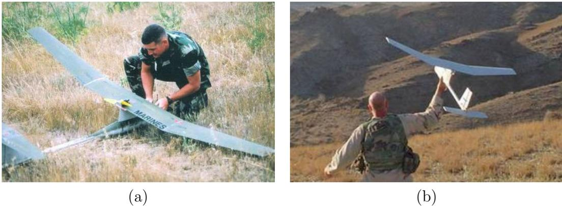
**Figure 36:** (a) Aerovironment Pointer UAV platform. (b) Aerovironment Raven UAV platform.
